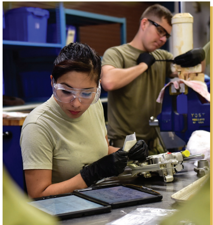
Senior Airman Joanna Escamilla, 4th Component Maintenance Squadron hydraulics technician, assembles an elevator actuator for an A-10 Thunderbolt. (Photo: Senior Airman Victoria Boyton)
